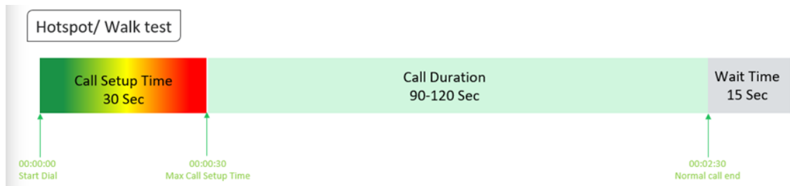
Figure-35: Voice test script for walktest/hotspot
