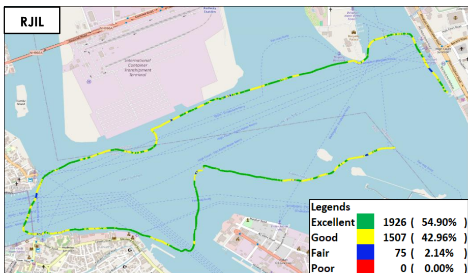
Figure-44: Signal strength auto-selection mode 5G/4G/3G/2G - RJIL
