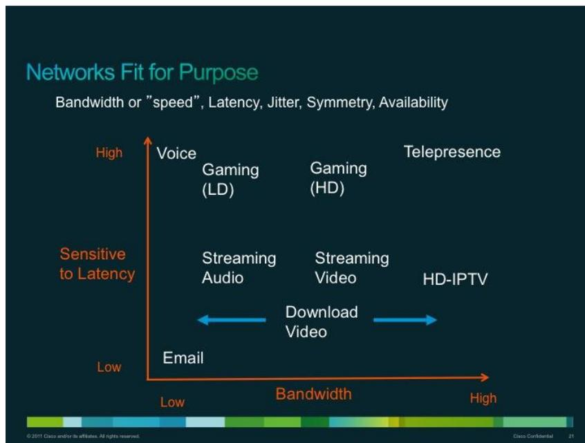
Network operators deploy tools to ensure that packets associated with latency- and jitter-sensitive applications arrive on time, and that the end user's experience is not disrupted by network congestion.
