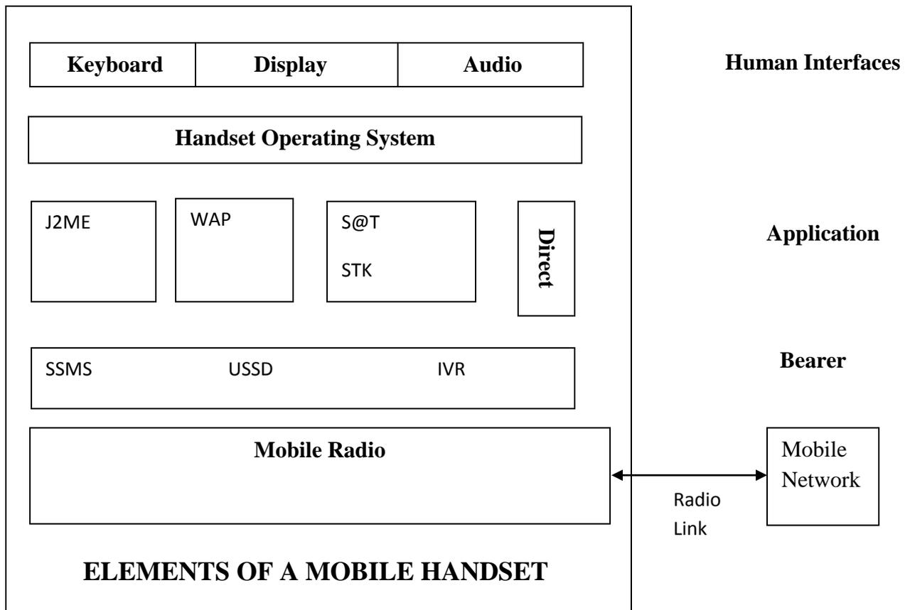
There are human interfaces of a mobile phone such as Keyboard, Display and Audio. The operating system ties all the elements of the handset together. Mobile radio communicates to the mobile network and has the capability to send SMS, USSD, voice data over the radio interface.
