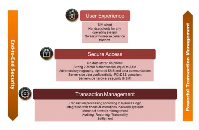
On the mobile front end, users are required to identify themselves with a PIN, which protects access to financial information and transactions. Secret keys only known to the SIM card and the service provider are used to encrypt and sign transaction data, further proving the identity of the user.
