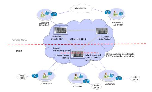
It is clear from above diagram that multiple OSPs can be hosted on a single India based HCC solution which will also cater to the regulatory requirement for each OSP, IP-PSTN restriction and Logs keeping. This solution will also ease out inspection agencies for audit purpose due to physical infrastructure in India and also a remote login facility can be provided from any OSP centre to monitor the CDRS, Logs, Call flow restrictions etc.
