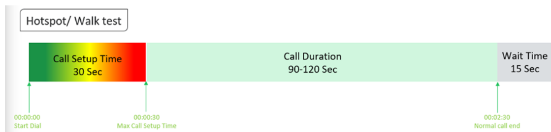
Figure-49: Voice test script for walktest/hotspot
