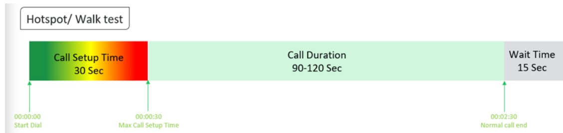
Figure-58: Voice test script for walktest/hotspot
