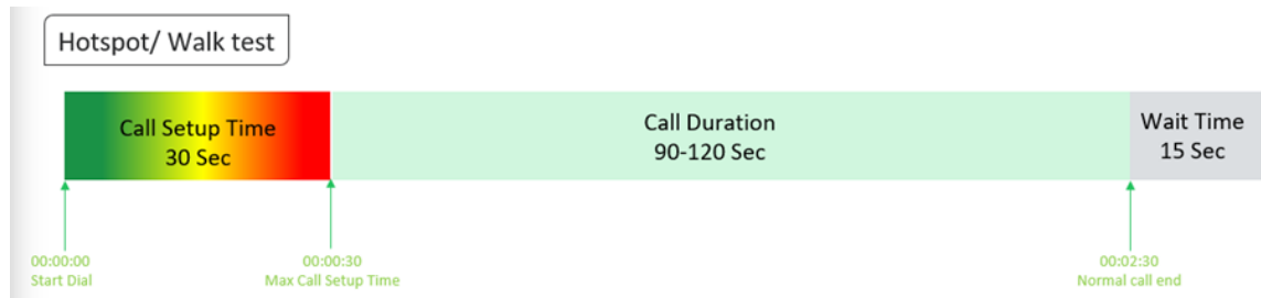
Figure-35: Voice test script for walktest/hotspot
