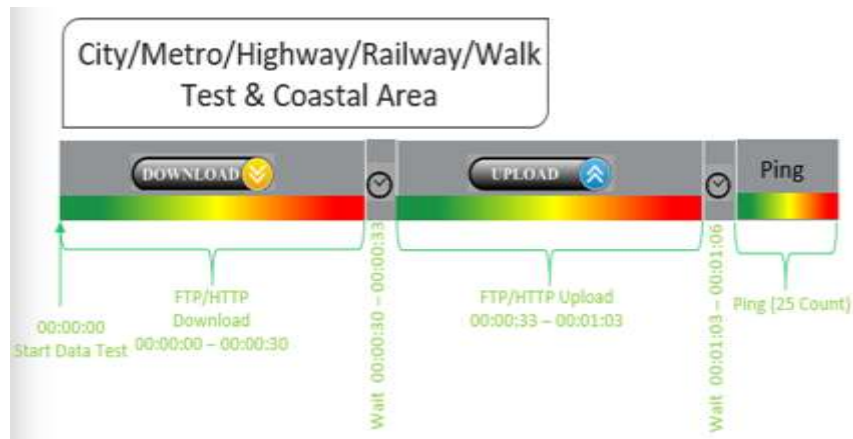
Figure-75: Data test script used in city/metro/railway/highway/walk test & coastal area
