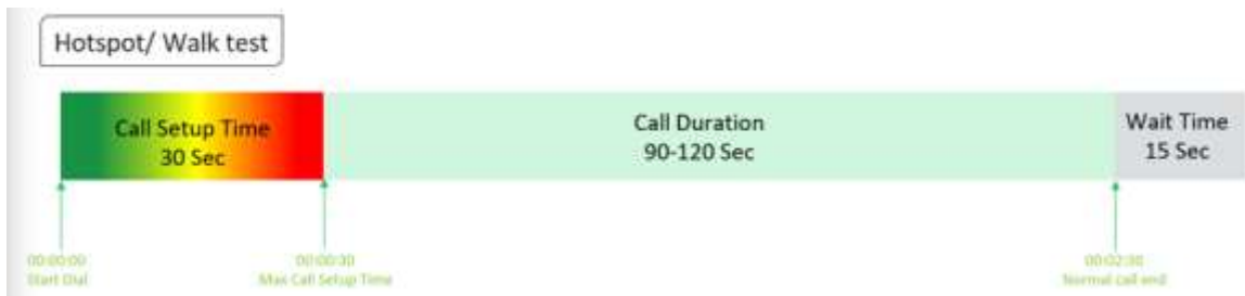
Figure-74: Voice test script for walktest/hotspot
