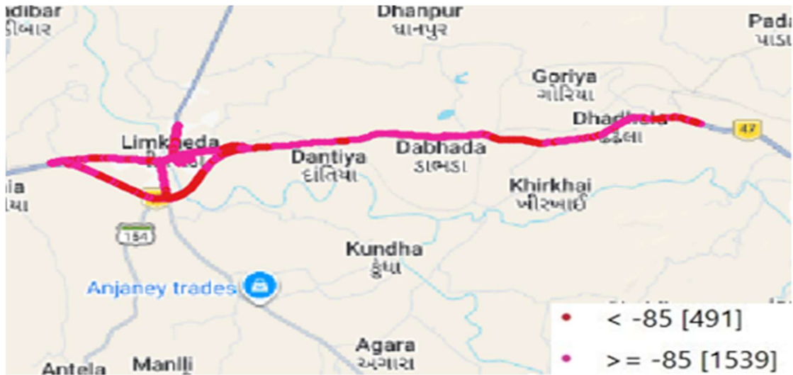
Figure-7: Signal strength 3G/2G network mode-AIRTEL
