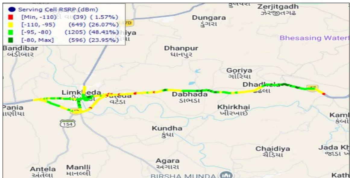
Figure-13: Signal strength auto-selection mode 5G/4G/3G/2G - VIL
