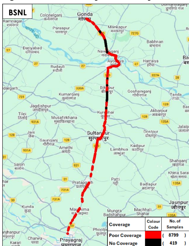
Figure-143: Poor coverage & no coverage locations in auto-selection mode (5G/4G/3G/2G) voice - BSNL.
