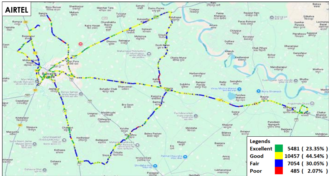
Figure-210: Signal strength auto-selection mode (5G/4G/3G/2G) voice - AIRTEL.
