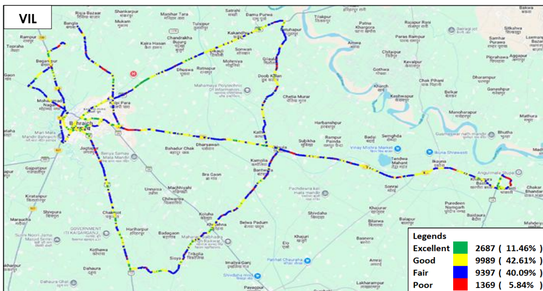
Figure-213: Signal strength auto-selection mode (5G/4G/3G/2G) voice - VIL.
