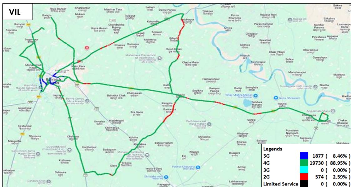
Figure-80: Serving technology plots in auto-selection mode (5G/4G/3G/2G) data - VIL.
