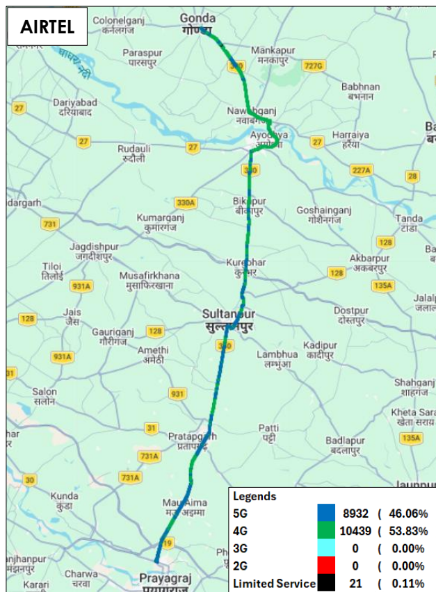
Figure-155: Serving technology plots in auto-selection mode (5G/4G/3G/2G) data - AIRTEL.
