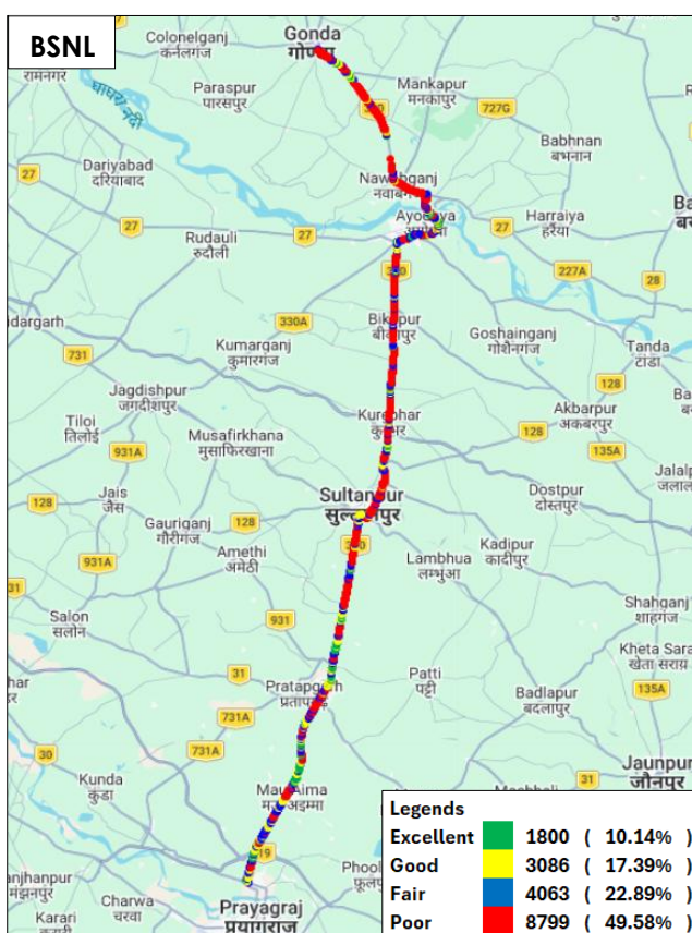
Figure-233: Signal strength auto-selection mode (5G/4G/3G/2G) voice - BSNL.
