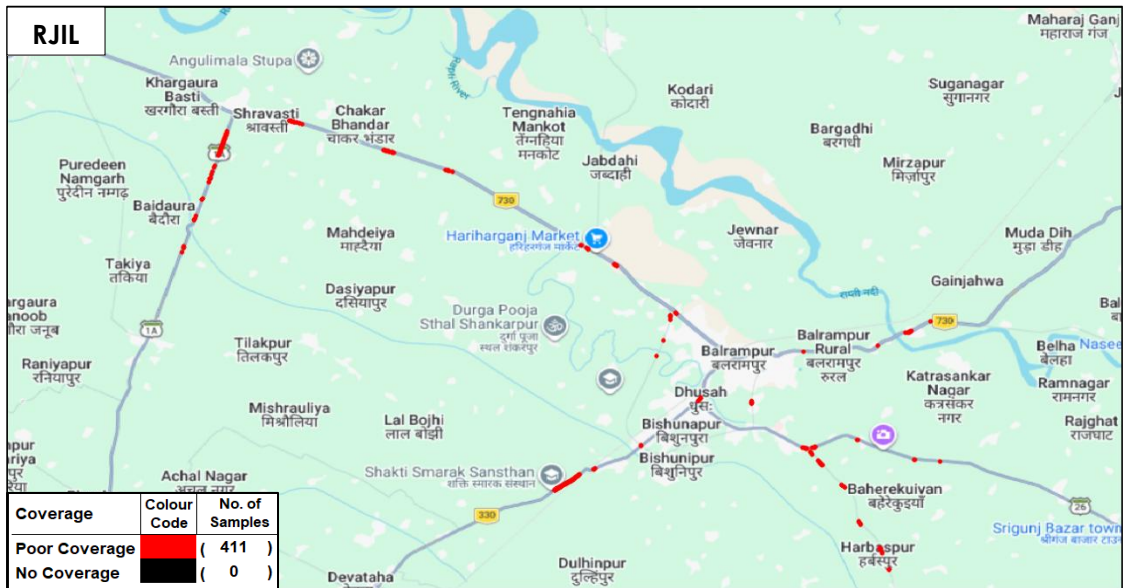
Figure-103: Poor coverage & no coverage locations in auto-selection mode (5G/4G/3G/2G) voice - RJIL.
