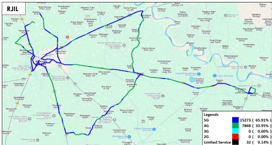
Figure-79: Serving technology plots in auto-selection mode (5G/4G/3G/2G) data - RJIL.
