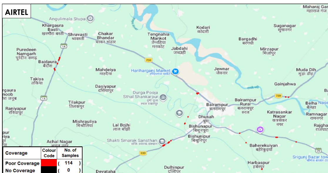
Figure-101: Poor coverage & no coverage locations in auto-selection mode (5G/4G/3G/2G) voice - AIRTEL.
