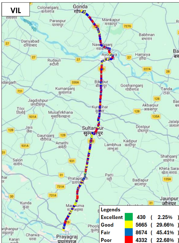
Figure-239: Signal strength auto-selection mode (5G/4G/3G/2G) data - VIL.
