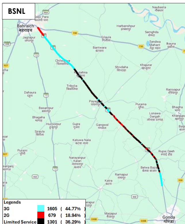
Figure-164: Serving technology plots 3G/2G network mode - BSNL.
