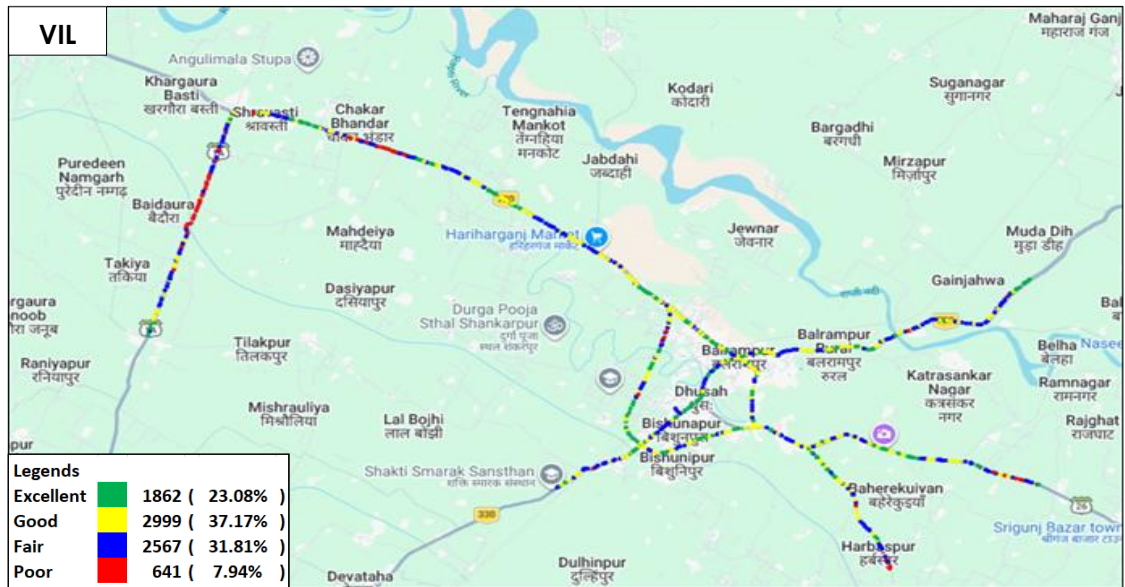
Figure-220: Signal strength 3G/2G network mode voice - VIL.
