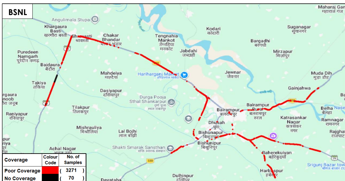
Figure-102: Poor coverage & no coverage locations in auto-selection mode (5G/4G/3G/2G) voice - BSNL.
