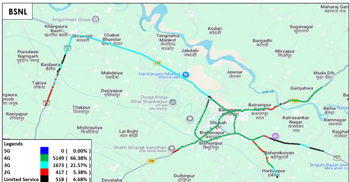
Figure-115: Serving technology plots in auto-selection mode (5G/4G/3G/2G) data - BSNL.
