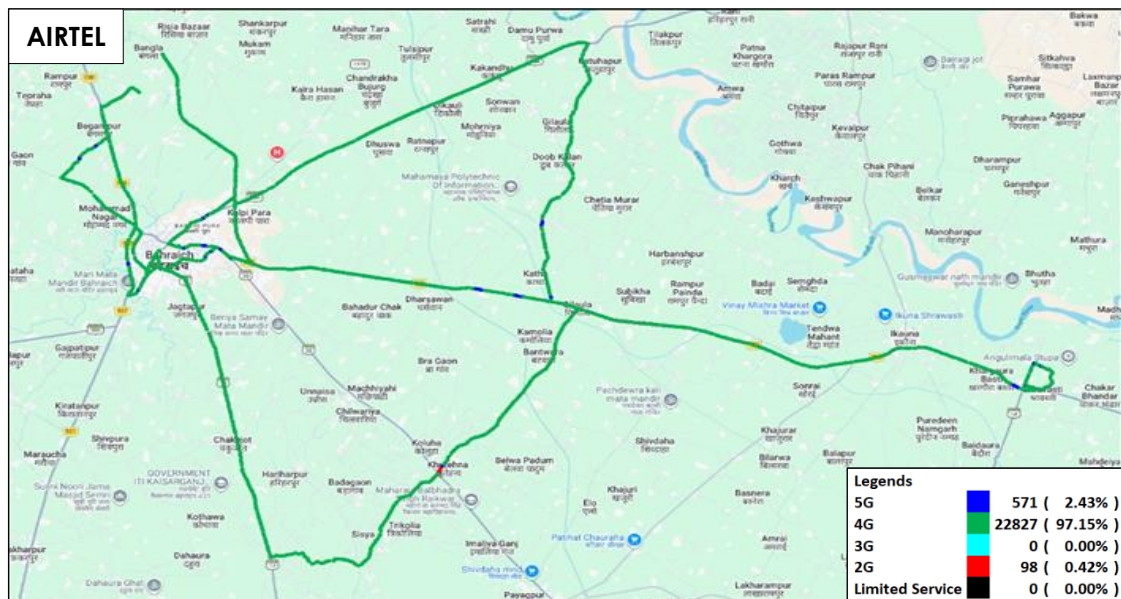
Figure-59: Serving technology plots in auto-selection mode (5G/4G/3G/2G) voice - AIRTEL.
