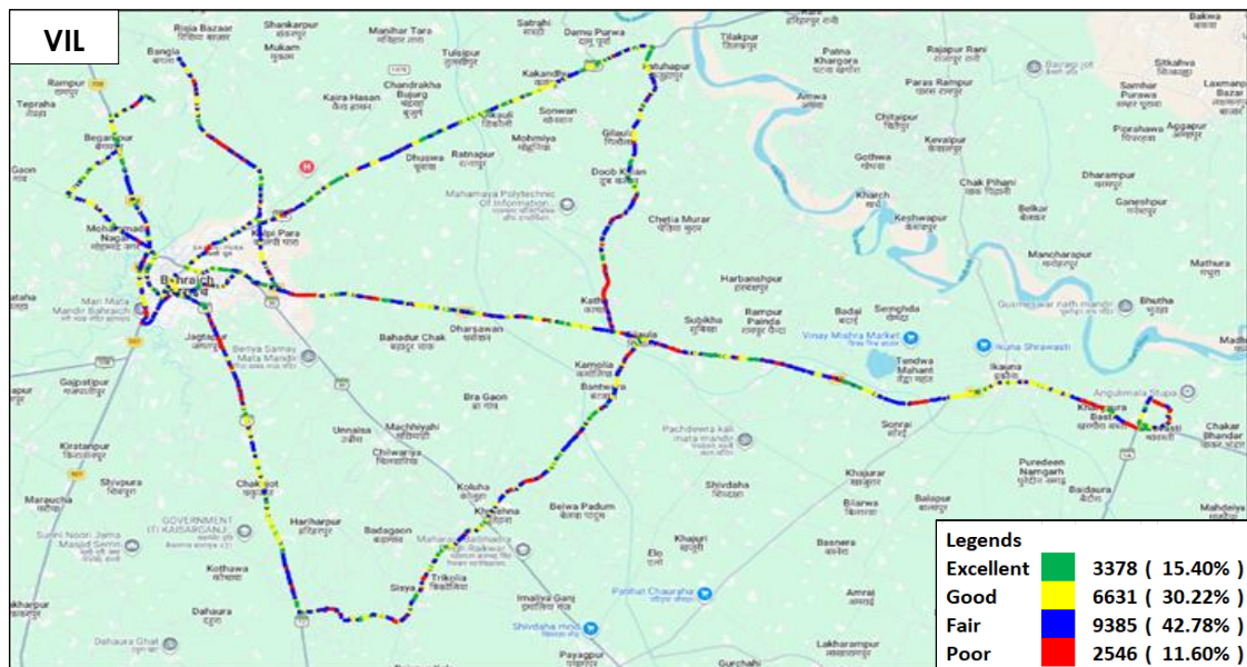
Figure-209: Signal strength 3G/2G network mode voice - VIL.
