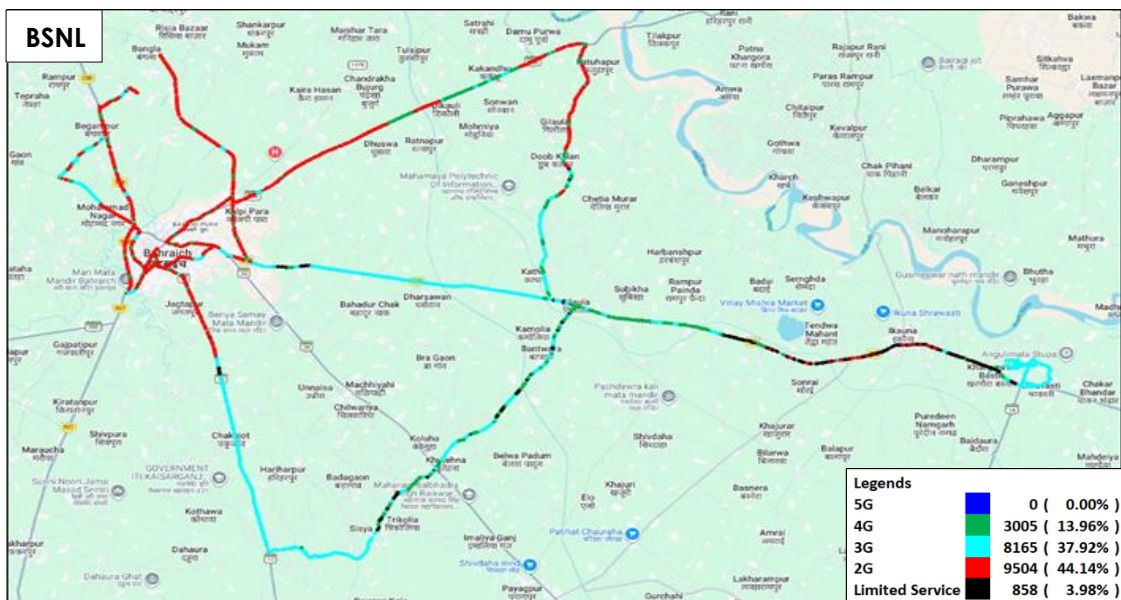
Figure-60: Serving technology plots in auto-selection mode (5G/4G/3G/2G) voice - BSNL.
