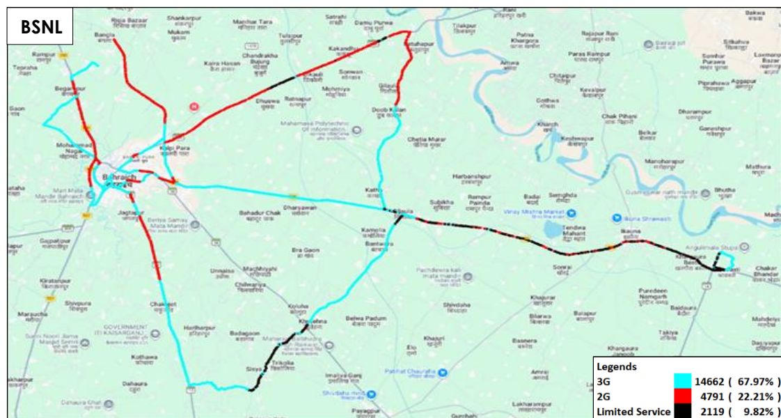
Figure-48: Serving technology plots 3G/2G network mode - BSNL.
