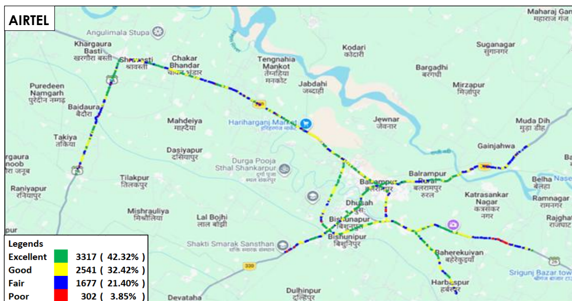
Figure-218: Signal strength 3G/2G network mode voice - AIRTEL.
