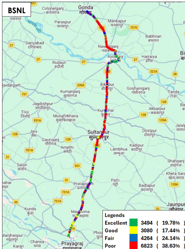
Figure-230: Signal strength 3G/2G network mode voice - BSNL.
