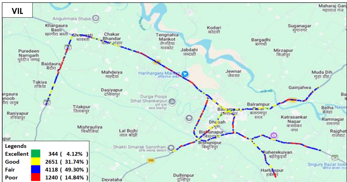
Figure-228: Signal strength auto-selection mode (5G/4G/3G/2G) data - VIL.
