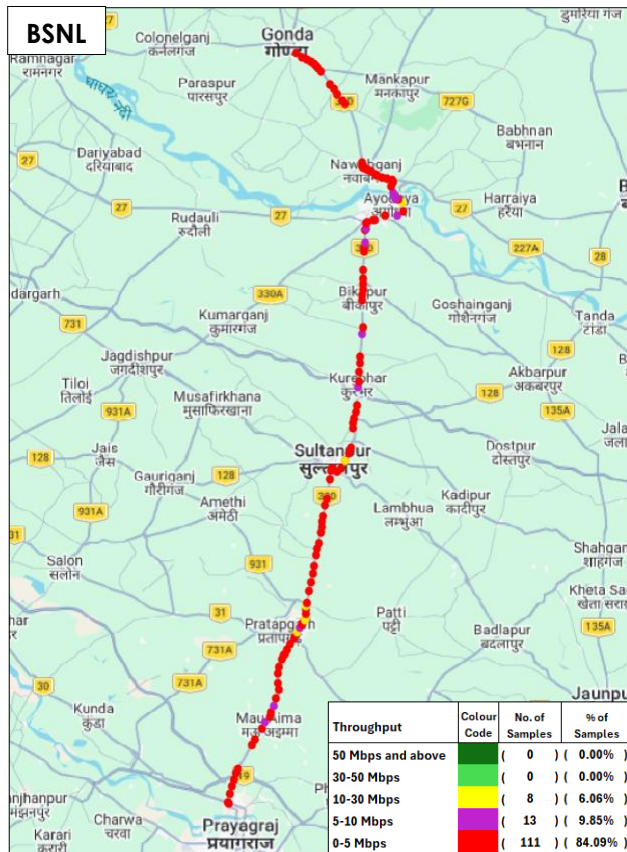
Figure-152: Upload throughput distribution auto-selection mode (5G/4G/3G/2G) - BSNL.
