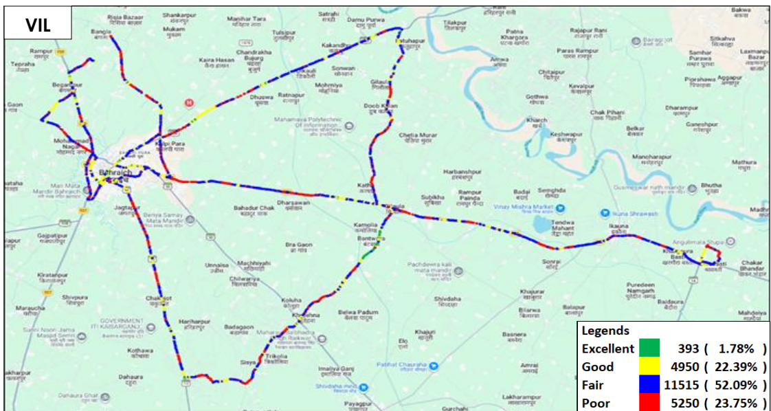
Figure-217: Signal strength auto-selection mode (5G/4G/3G/2G) data - VIL.
