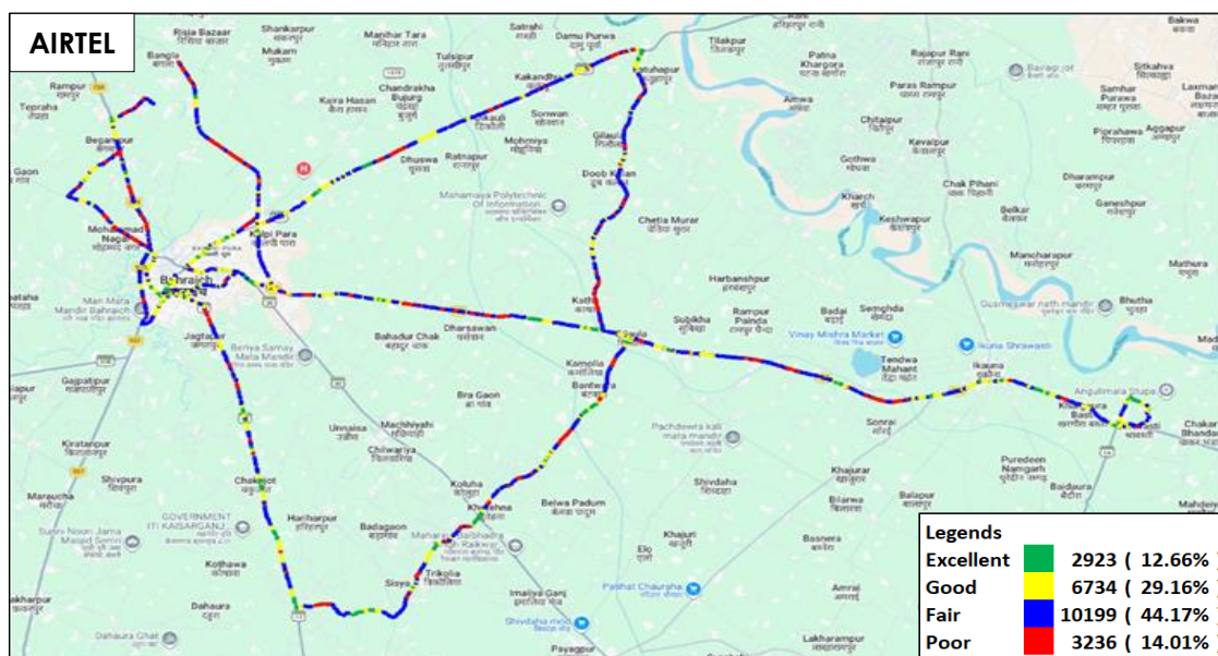
Figure-214: Signal strength auto-selection mode (5G/4G/3G/2G) data - AIRTEL.
