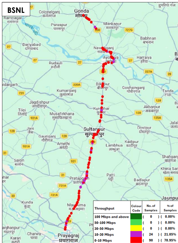
Figure-148: Download throughput distribution auto-selection mode (5G/4G/3G/2G) - BSNL.
