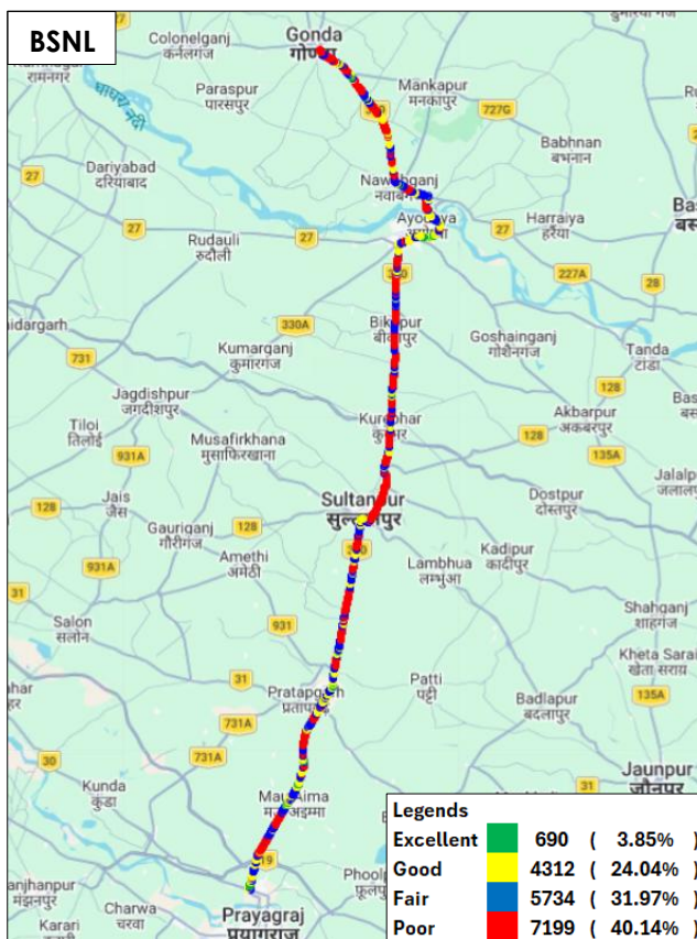
Figure-237: Signal strength auto-selection mode (5G/4G/3G/2G) data - BSNL.
