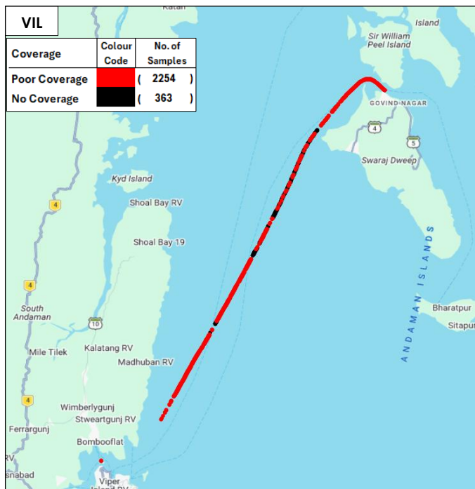
Figure-69: Poor coverage & no coverage locations in auto-selection mode (5G/4G/3G/2G) voice-VIL.
