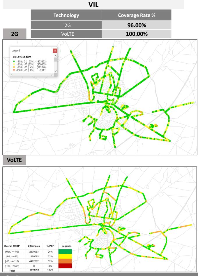
For measuring voice quality, as per the QoS norms, RxQual <=5 for GSM TSPs, EcNo >= -14 dBm for 3G TSP sand SINR >0 in case of VoLTE is considered to be good, where as quality beyond this benchmark is considered to be bad. The benchmark should usually be  $\geq$  95%.
