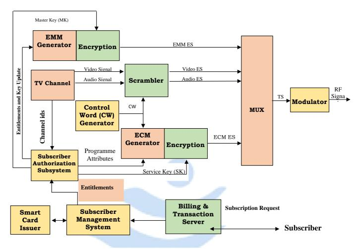
Figure 8: The basic structure of CAS at the transmitter side in an encrypted TV Broadcasting Service
