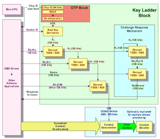
Figure 12: Key Ladder Block Diagram<sup>25</sup>
