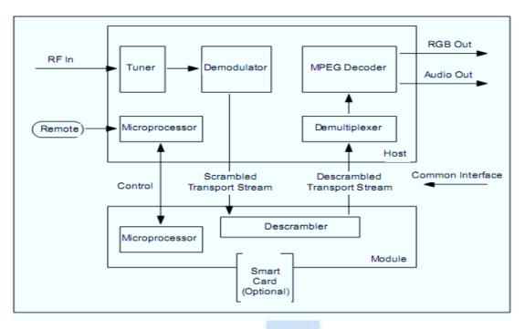
Figure 7: Functional Block Diagram of a STB
