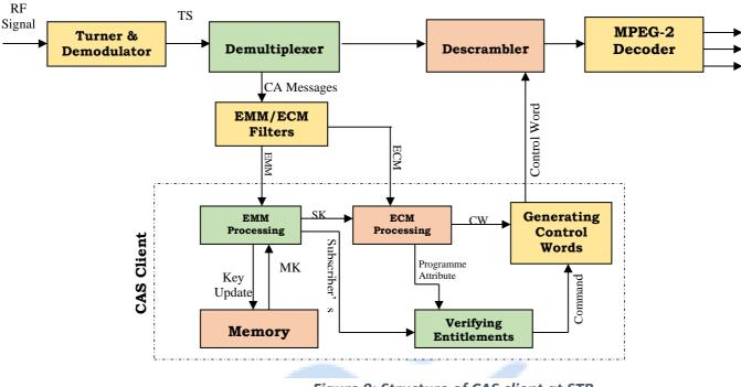
Figure 9: Structure of CAS client at STB
