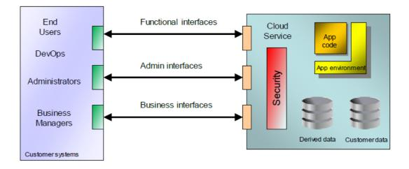
Figure 3.2: Elements of interoperability for Cloud Services<sup>16</sup>
