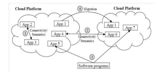
Figure 3.1: Types of interoperability between various applications on Cloud<sup>14</sup>
