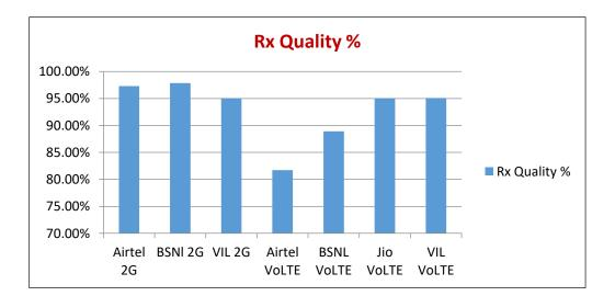
For measuring voice quality, as per the QoS norms, RxQual <=5 for GSM TSPs, EcNo >= -14 dBm for 3G TSP sand SINR >0 in case of VoLTE is considered to be good, where as quality beyond this benchmark is considered to be bad. The benchmark should usually be  $\geq$  95%.
