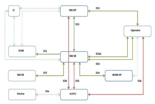
Figure 1.1: Remote Provisioning Architecture for M2M eSIM [Source: GSMA SGP.02<sup>6</sup>]
