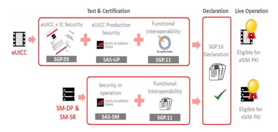
Figure 2.1: GSMA's security compliance framework for eSIM
