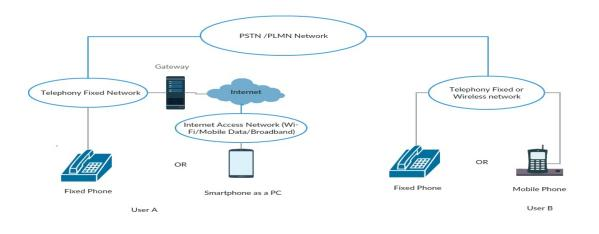
Figure 4: Hybrid/Mix of Fixed line and Internet Telephony
