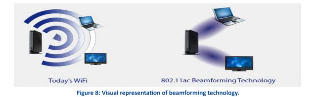
of al lot of information between the users and antennas on a massive MIMO arrays by choreographing the packets' movements and arrival time. Beamforming and the devices that support beamforming work under the IEEE 802.11ac specification.
