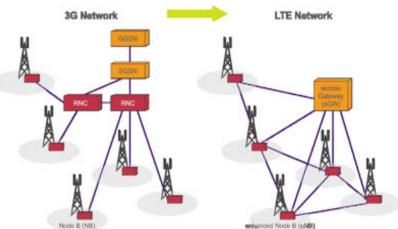
Figure 2: Evolution from UMTS technology used in 3G to LTE used in 4G
