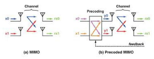
Figure 7: Difference between MIMO and Precoded MIMO
