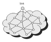
Figure 4 Flat network architecture
