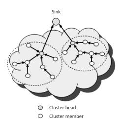
Figure 5 Multihop clustering architecture
