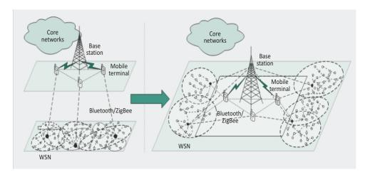
Figure 2 Converged network architecture for MCN and WSN
