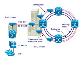
Figure 2 Network extension and fibre complement through FSO
