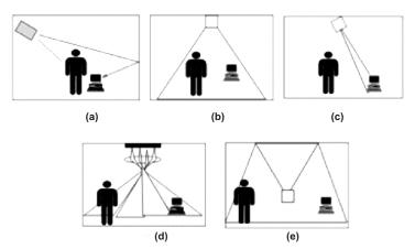
Figure 11 (a) Diffuse system. (b) Wide LOS system (c) Narrow LOS system with tracking (d) Narrow LOS system using multiple beams (e)Quasi diffuse system
