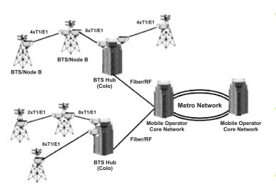
Figure 4 Backhaul connection through FSO
