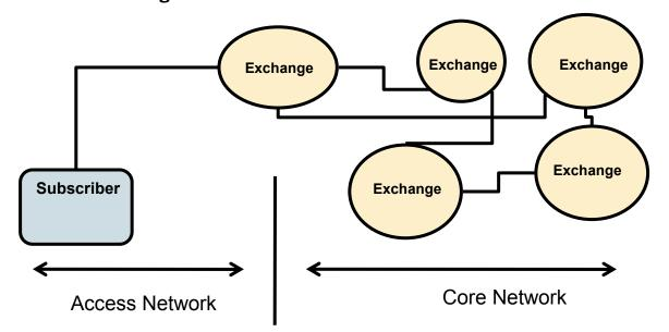
Figure 3.1: Schematics of Broadband network
